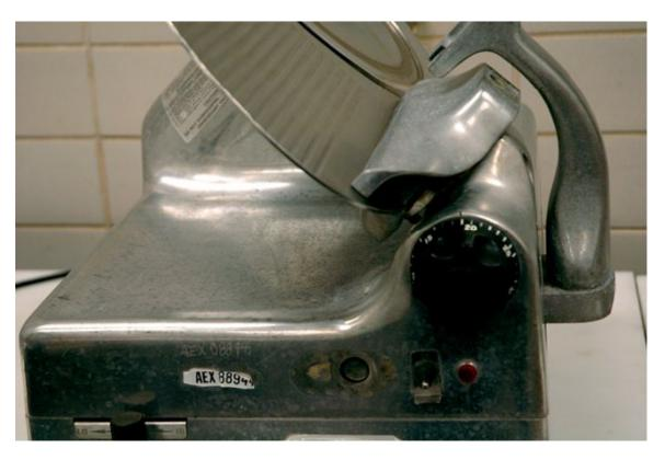
A slicer blade with grime and black residue under the blade. The blade can be contaminated with *Lm* and spread to the product that is sliced. The slicer handle, controls, and seals may also be contaminated, as these areas may not be frequently cleaned.
